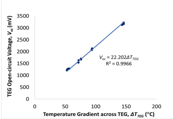
Figure 10: Open-circuit voltage versus temperature difference across TEG.
