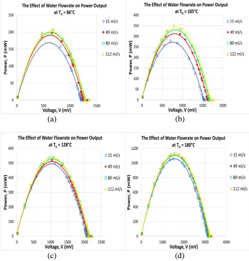
Figure 8: The effect of water flowrate on power output at different TEG hot-side temperatures (a)  $T_h = 86^\circ\text{C}$ , (b)  $T_h = 105^\circ\text{C}$ , (c)  $T_h = 128^\circ\text{C}$ , and (d)  $T_h = 180^\circ\text{C}$ .
