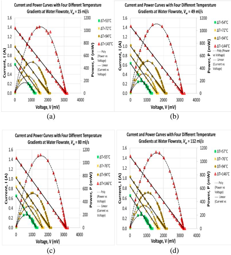
Figure 9: Current and power curves with four different temperature gradients across TEG at different water flowrates (a)  $V_w = 15$  ml/s, (b)  $V_w = 49$  ml/s, (c)  $V_w = 80$  ml/s, and (d)  $V_w = 112$  ml/s.
