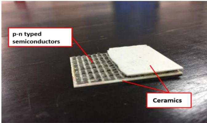
Figure 1: Thermoelectric Generator
