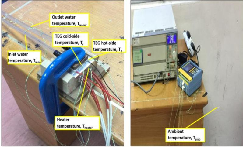
Figure 6: Six different locations of thermocouples
