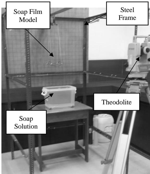
Figure 4: Experiment setup for soap film model.
