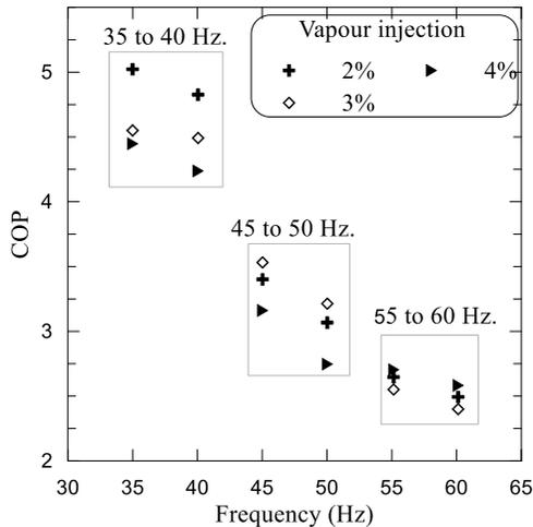
Figure 10: COP versus compressor power supply frequency for different vapor injection ratios.
