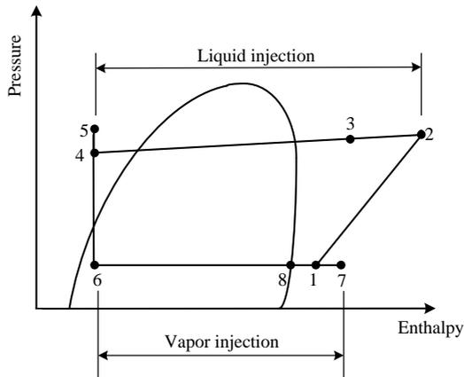
Figure 1 (b): Schematic diagram of the vapor compression cycle with liquid and vapor injection processes
