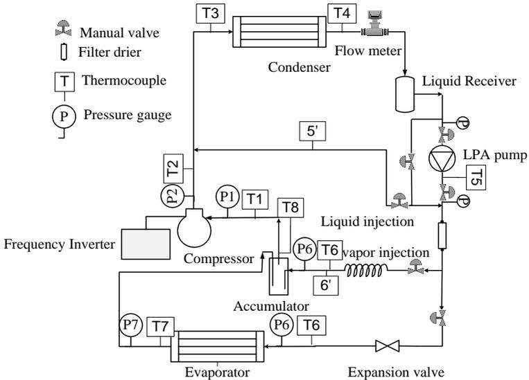
Figure 1 (a): Schematic diagram of the vapor compression cycle with locations of the refrigerant injection devices.
