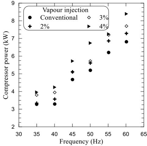
Figure 9: The variation of the compressor power with compressor power supply frequency for different vapor injection ratios.
