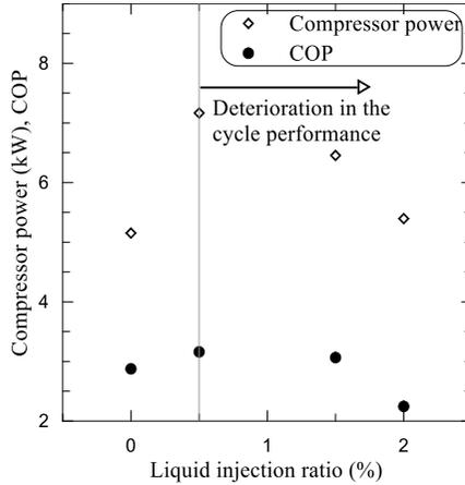
Figure 6: The effect of liquid injection on the compressor power and cycle COP.
