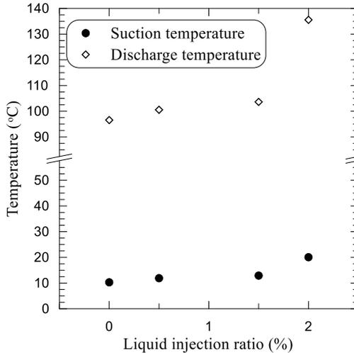
Figure 5: The variation of suction and discharge temperatures with the liquid injection ratio.
