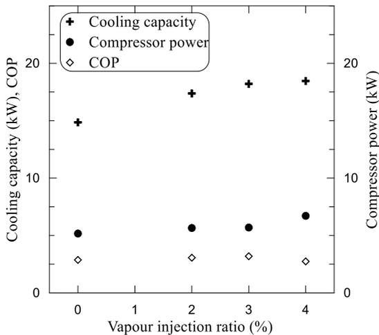
Figure 4: The effect of vapor injection ratio on the system performance.
