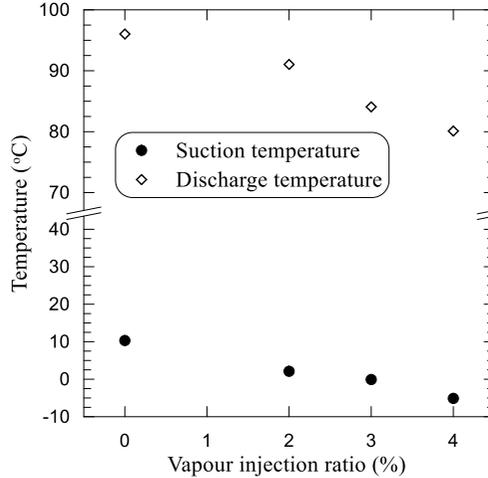
Figure 3: The variation of suction and discharge temperatures with the vapor injection ratio.
