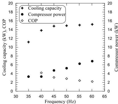
Figure 7: The effect of power supplied in frequency on the cycle performance.
