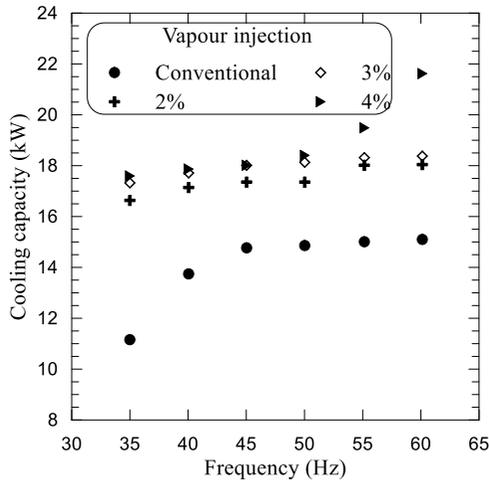
Figure 8: The variation of the cooling capacity with compressor power supply frequency.
