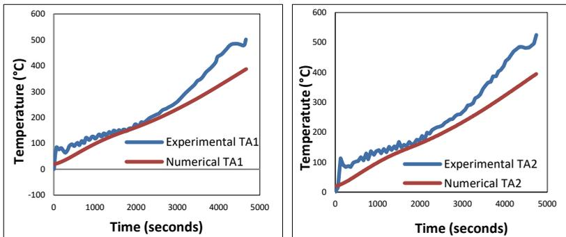
Figure 3: Comparison between experimental and numerical modeling of thermocouples labelled as TA1 and TA2 of CSB
