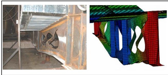
Figure 8: Comparison between predicted maximum vertical deflection using ABAQUS simulation failure mode against the experimental test of CSB under fire loading and static loading [15].
