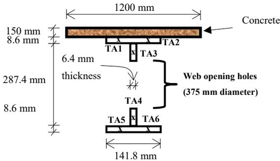
Figure 2: Thermocouples location viewed from cross section A-A of the composite concrete slab-cellular steel beam [6,15]
