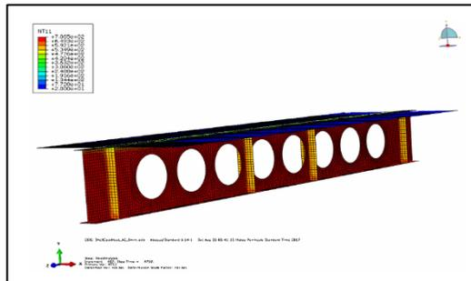
Figure 6: Predicted maximum temperature profile of CSB model at elevated temperature (4800 seconds)
