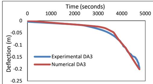
Figure 7: Measured and predicted vertical deformation in the middle and centered of CSB
