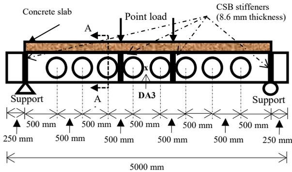
Figure 1: Composite concrete slab-cellular steel beam [6,15]
