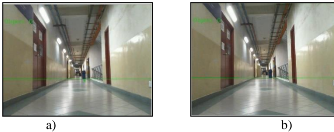
Figure 11. a) The moving object detected until 13meter distance from webcam b) Show that moving object when reach 15meter distance are not detected, the object counter also does not increase
