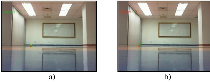
Figure 9. a) At 10m, the moving object showing that it is fairly detected. b) After the moving object crossed the green lines, the object is shown count from 1 to 2.
