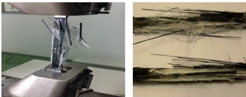
Figure 11: Failure mode of delamination experienced by Hybrid B
