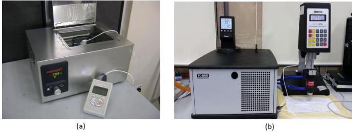
Figure 1 : (a)Thermal conductivity and (b) viscosity measurement instruments
