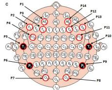
Figure 2: Emotiv Epoch Neuroheadset Electrode Placement
