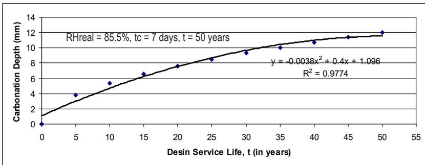
Figure 5: Design service life vs. Carbonation depth
