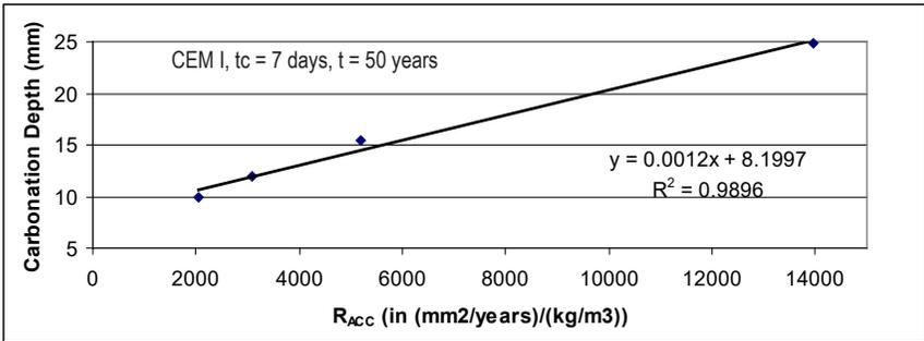
Figure 6: RACC vs. Carbonation depth
