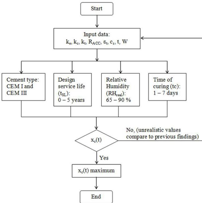
Figure 3: Flowchart for concrete carbonation depth calculation
