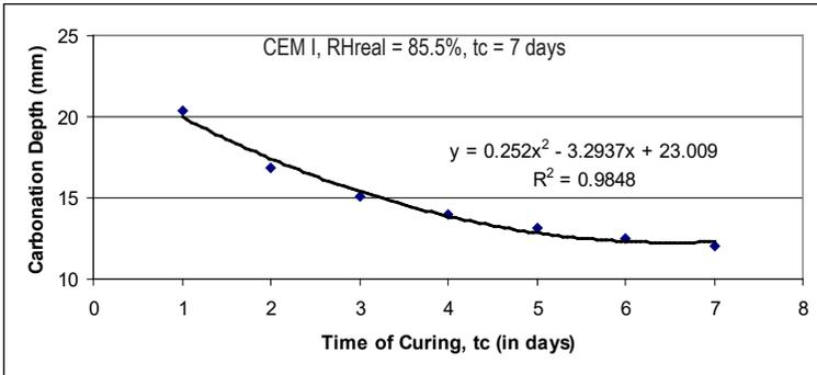
Figure 4: Time of curing vs. Carbonation depth
