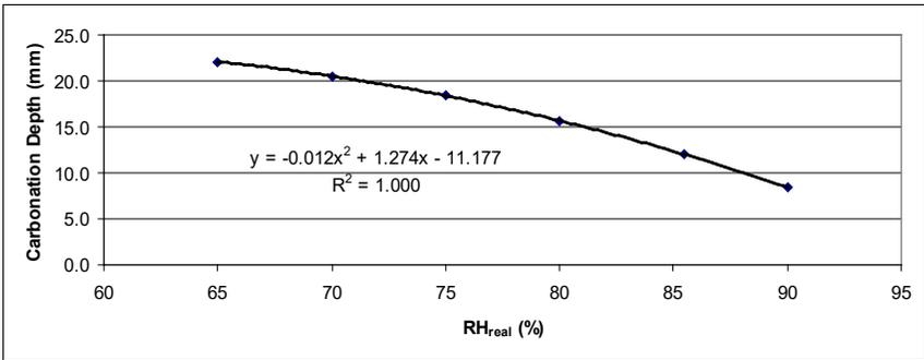
Figure 7: RH<sub>real</sub> vs. Carbonation depth
