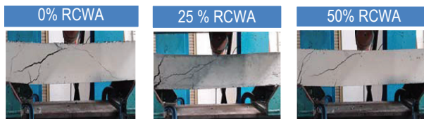
Figure 4: The Effect of RCWA to the Beams Deflection Behaviour
