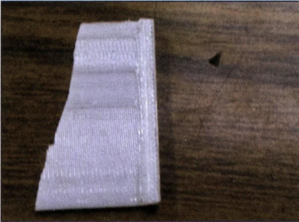
Figure 11: Broken cutting edge showing the layers of material
