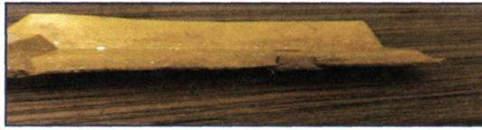
Figure 9: Failure of original blade due to obstacle impact
