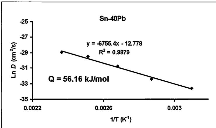
Figure 11: Arrhenius Plot of the Cu<sub>6</sub>Sn<sub>5</sub> Intermetallic Layer Growth for the Sn-40Pb/Cu System
