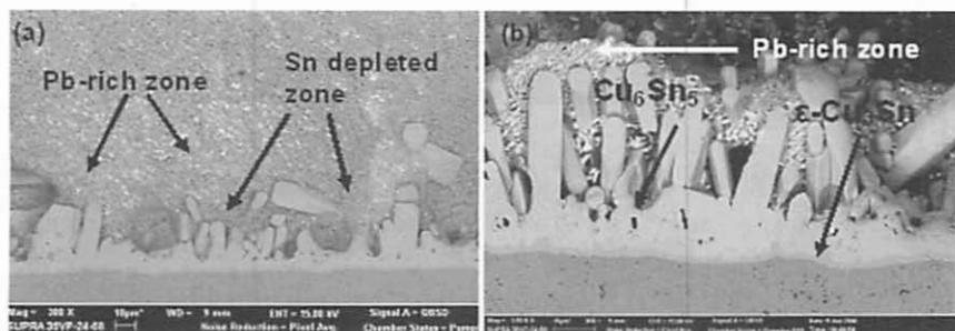
Figure 7: The Reaction between Sn and Cu Creates (a) a Sn Depleted Zone and Results in (b) the Cu<sub>6</sub>Sn<sub>5</sub> Intermetallic Penetration into the Pb-rich Zone. Both Images are for Samples Aged at 150°C for 100 Hours
