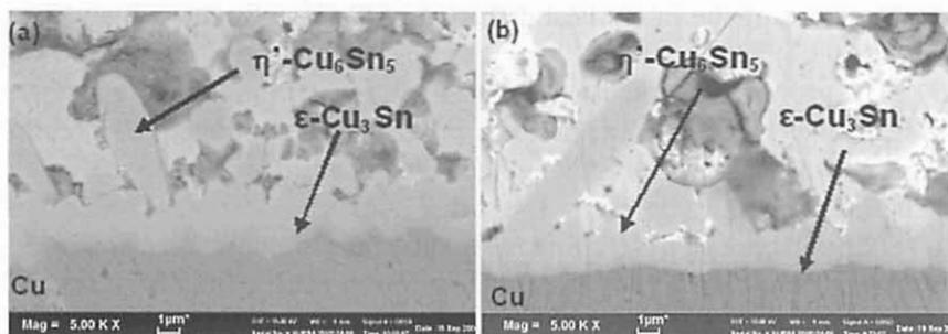
Figure 5: The Formation of the IMC Layer between the Sn-40Pb and Cu Substrate for Samples Isothermally Aged at  $75^\circ\text{C}$  for (a) 100 and (b) 700 Hours
