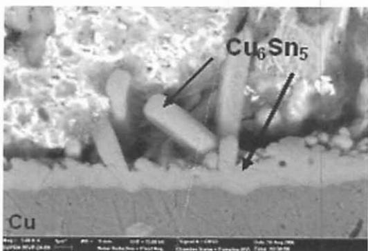
Figure 4: IMC Layer Formed between the Sn-40Pb and Cu Substrate Isothermally Aged at 50°C for 500 Hours
