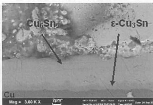
Figure 9: IMC Layer Formed between Sn-40Pb and Cu Substrate Isothermally Aged at 150°C for 700 Hours
