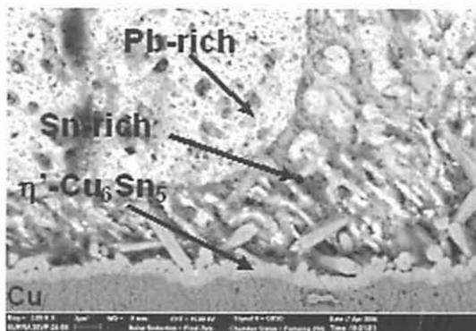
Figure 3: As-soldered IMC Layer between the Sn-40Pb and Cu Substrate
