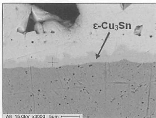
Figure 6: The Manifestation of the  $\epsilon$ - $\text{Cu}_3\text{Sn}$  Below the  $\text{Cu}_6\text{Sn}_5$  IMC for a Sample Aged at  $150^\circ\text{C}$  for 100 Hours
