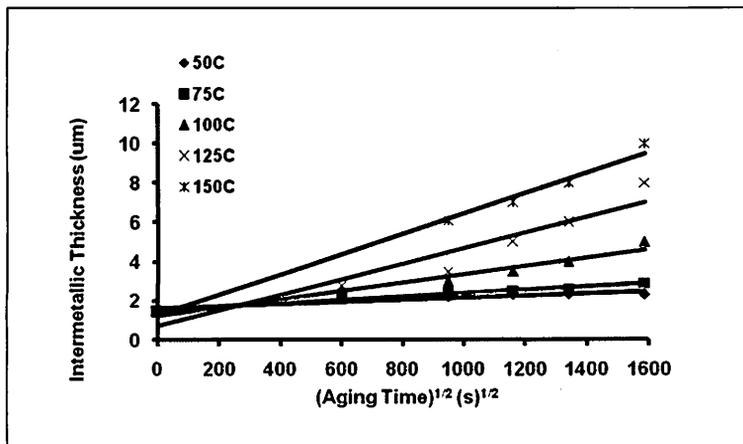
Figure 10: The Relationship between Cu<sub>6</sub>Sn<sub>5</sub> Intermetallic Thickness and Aging Time,  $t^{\frac{1}{2}}$
