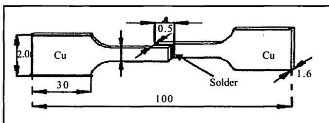
Figure 1: Single Lap Dog-bone Shape (All Dimensions in mm)
